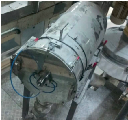
Model FTIC-0800 centrifugal sieve shaker with 300µ mesh, for the sieving of a mixture of flours on a continuous bagging line.
