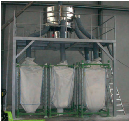
Separation sieving for BIG BAG loading using FTI-1200 sieve shaker, through three separations on a PET recycling line, with a rate of more than 2,000 Kg/hour.
