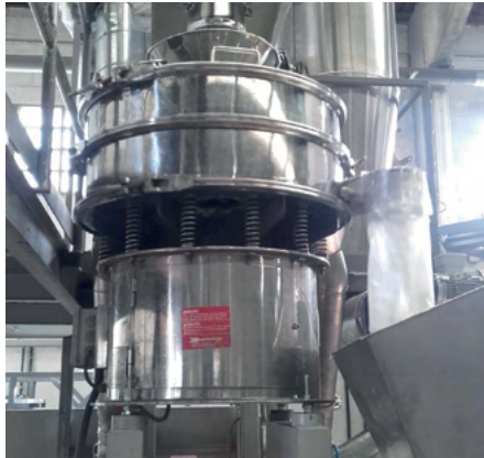
FTI-0800 circular sieve shaker on silo unloading line, with #1.2mm mesh for the separation of spices (thyme, cinnamon) at a rate of 1,000Kg/hour.
