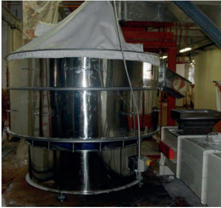
Sieving application for the separation of particles in suspension in the form of powder (150µ). Sieve shaker adapted to fluid bed line.
