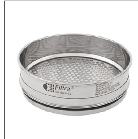
Stainless steel sieve with round perforated plate.
