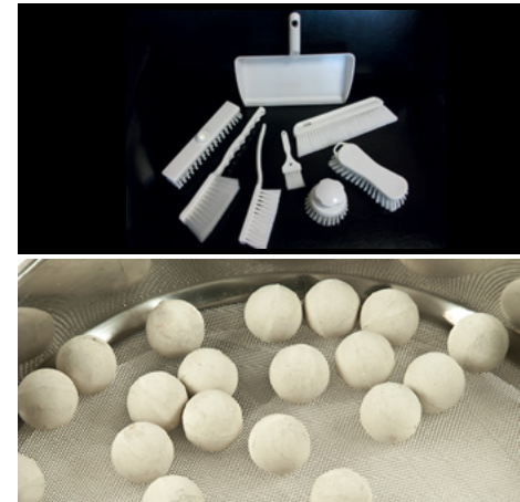
1. Cleaning brushes for sieves. 2. Food balls used to open the mesh of sieve.
