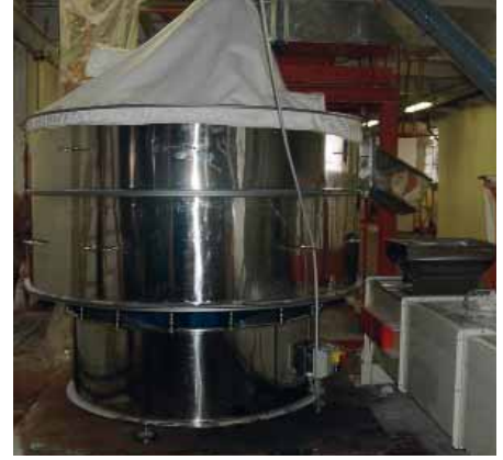
Sieving application for the separation of particles in suspension in the form of powder (#150µ). Sieve shaker adapted to fluid bed line.
