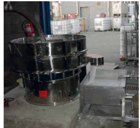
Model application of the FTI-1200 for viscous products (glues), to T eliminate impurities on a production line.
