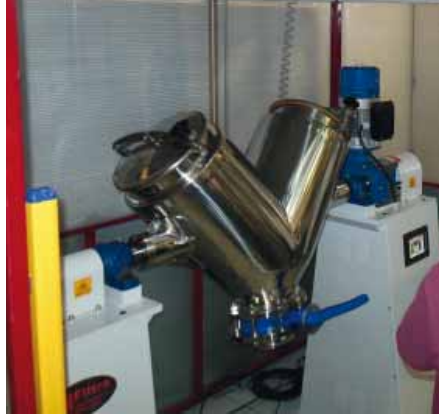
FTIMV- 100L UVE industrial mixer, integrated control panel with programmable automaton and touchscreen to access editable programme menu. Features optical security barriers.
