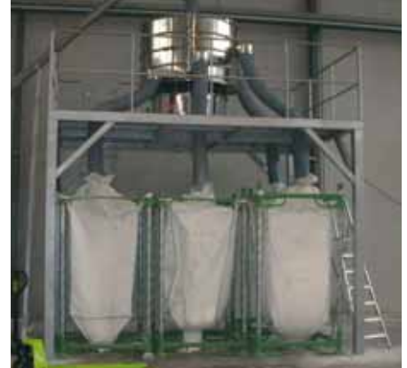
Separation sieving for BIG BAG loading using FTI-1200 sieve shaker, through three separations on a PET recycling line, with a rate of more than 2,000Kg/hour.
