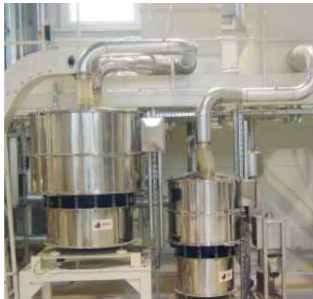
Example of applications for sieving on a line with FTI-1200 and FTI-0550 sieve shakers working in cascade.
