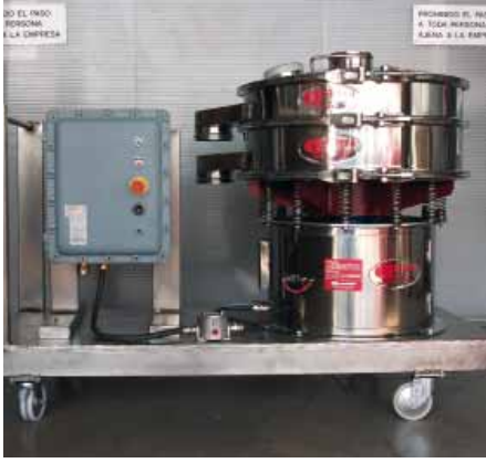
Model FTI-0800ATEX Sieve Shaker Zone 22 3D T4 with #125µ mesh, installed with electrical control panel on a moveable surface, according to the client's specifications.
